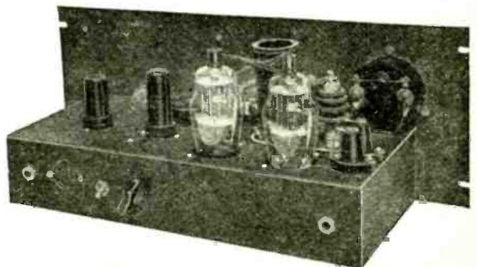
Rear view of the unit. Note shunt across meter and jacks for keys.
