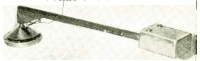
The completed pickup. Tone-arm weight is compensated by a spring.
